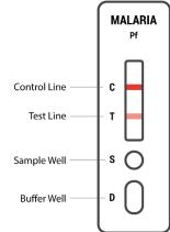
Absence of a coloured band in the test region indicates a nonreactive test result. A procedural control line should always develop at the 'C' region to indicate that the test has been carried out correctly.
